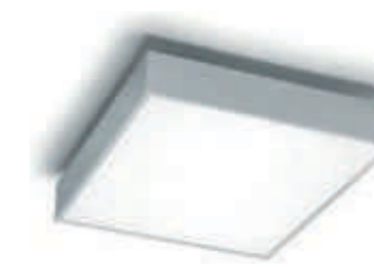
LED-Anbauleuchte direkt 5489281 1110lm 18W L/B300xH80mm 5489272 1800lm 30W L/B430xH80mm 5489275 4410lm 70W L/B600xH80mm
